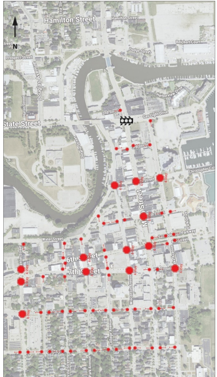
Figure 22: Stop controls after removing one-way operation.
