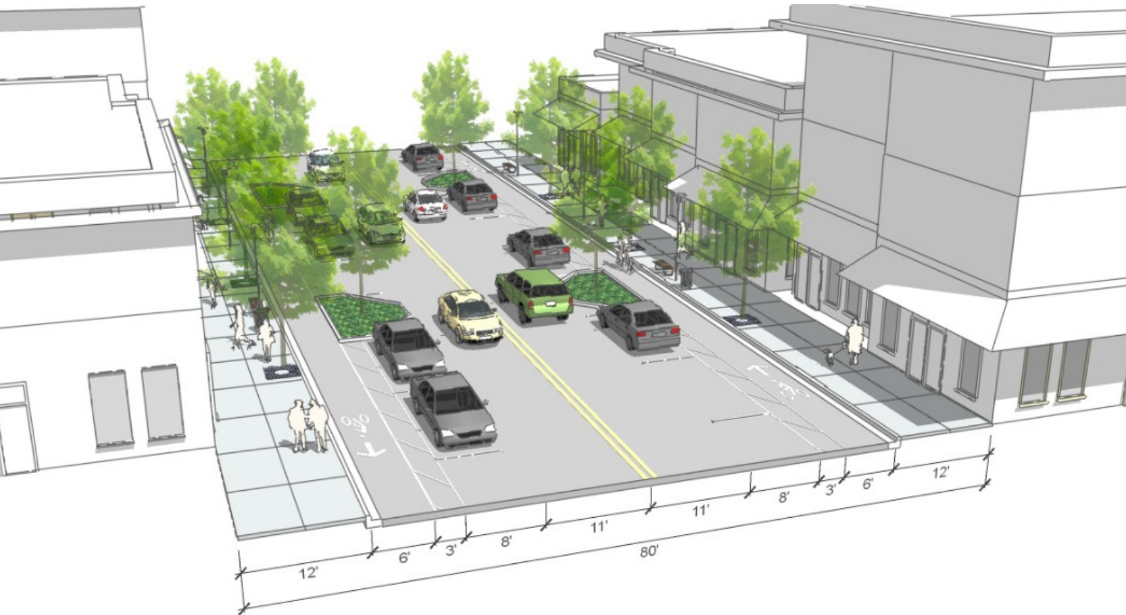
Figure 6: Interim Main Street retrofit.
