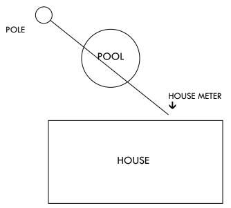
THERE MUST BE A MINIMUM <u>10 FOOT CLEARANCE</u> FROM SIDE WALL OF SWIMMING POOL TO POWER LINES
